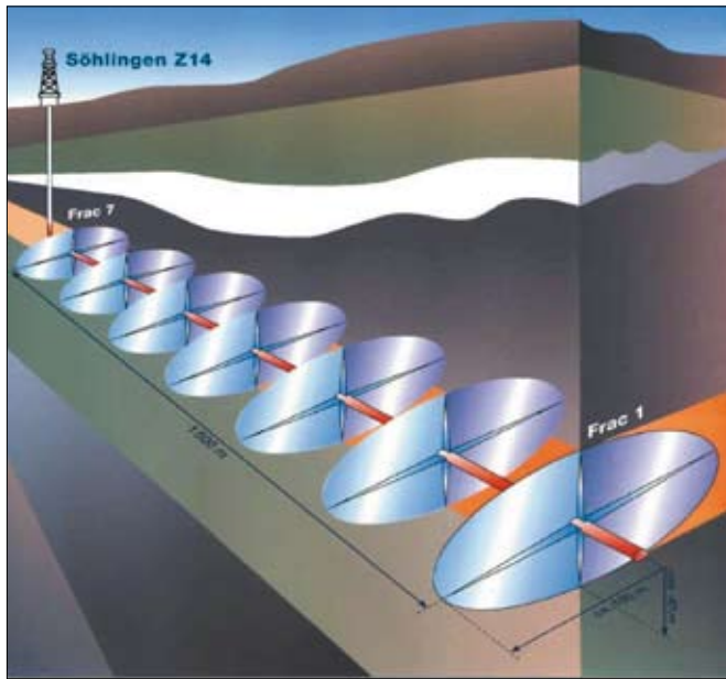
Fig. 5: The use of multiple frac treatment in horizontal drilling at Söhlingen Z 14 to lead to economic natural-gas extraction from Rotliegend sediments [8]
